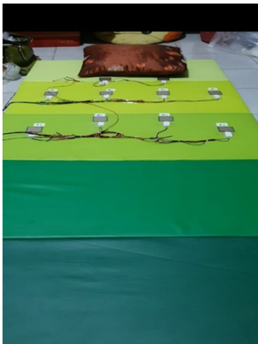
Figure 16 Bed mattress with force sensors installed.
