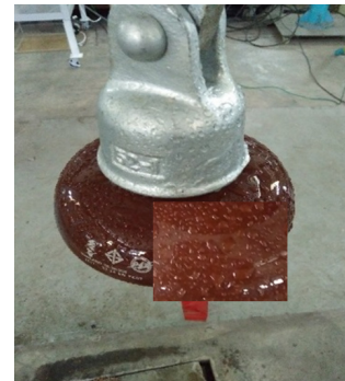
Figure 15: Test clean insulator, HC=2.
