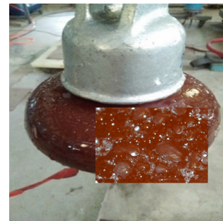
Figure 16: Test kaolin pollution, HC=5.
