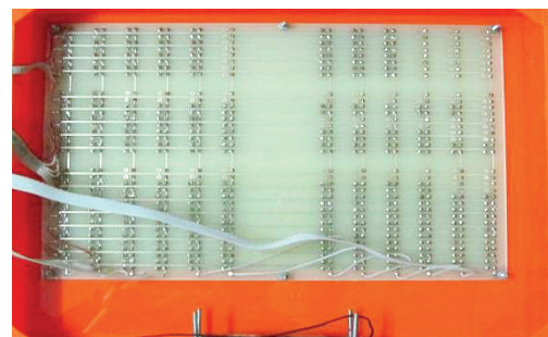
Figure 4 Wiring on the back side of the switchmatrix in the Braille learning set.
