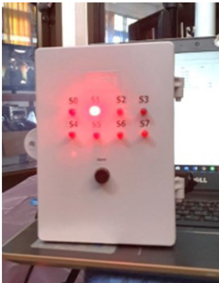
Figure 14 Example of the display represented the status of sleep through an LED set. For example, this Figure shows the position where the patient is lying on their back, the LED corresponding to (S1) will illuminate.
