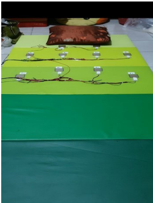
Figure 16 Bed mattress with force sensors installed.
