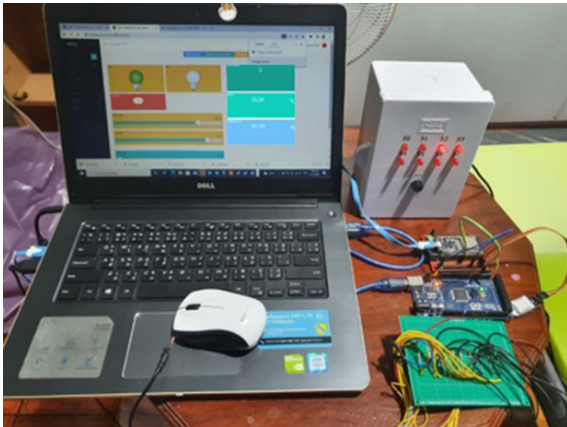
Figure 15 Developed smart bed system for monitoring sleep position.
