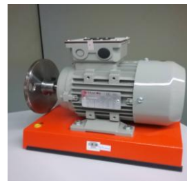
Fig. 5 The motor with unbalanced mass assembly
