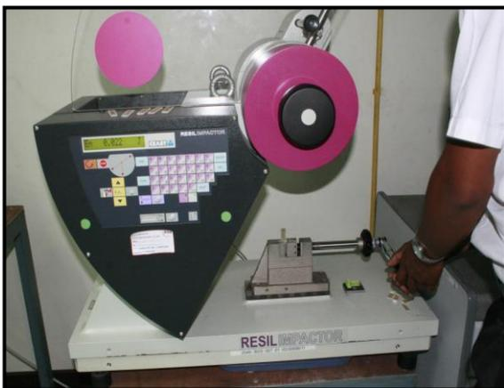
Figure 8: Izod impact test set-up
