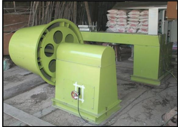
**Figure 3:** Automatic fiberglass winding machine [3]
