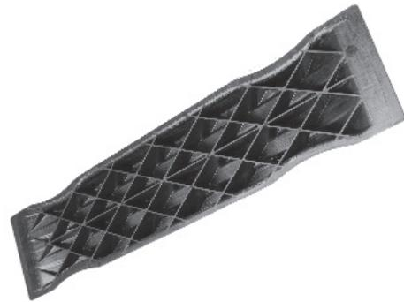
**Figure 4:** Side impact protection beam made of an organic sheet and a ribbed structure in an injection molding process [12].
