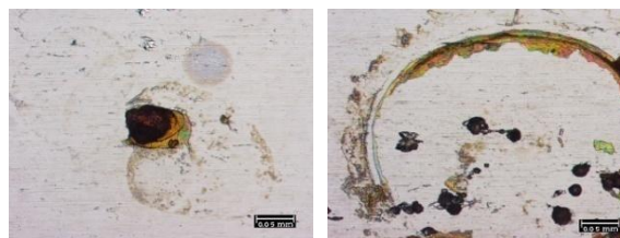
a) Industrial environment b) Marine environment Figure 8: 430 BA exposed for 9 months, 200x
