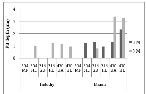
Figure 2: Pit depths of the specimens exposed for 3 and 9 months
