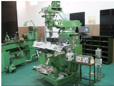
Figure 4: MAF setup in a milling machine
