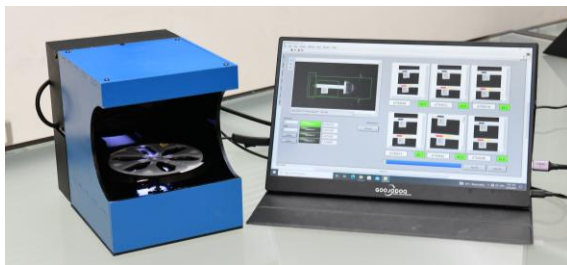
Figure 6: Automated hematocrit (Hct) reading system with an integrated image processing module developed in the LabVIEW environment. The system comprises a custom optical detection unit (left) for capturing images of microfluidic blood collection
