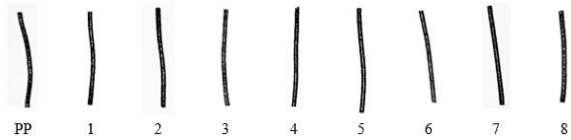
Figure 2: Manufactured filaments of r-PP and r-PP/Al composites.
