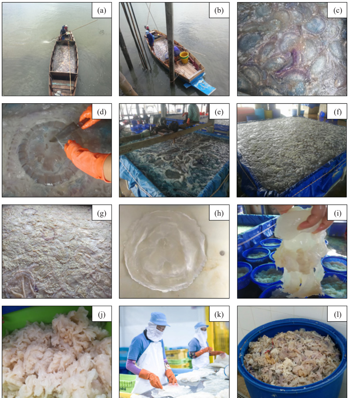
Figure 1: Production of salted jellyfish Lobonema smithii in Thailand. (a) Fresh jellyfish; (b) The transport of caught jellyfish to the land; (c) Jellyfish Lobonema smithii ; (d) The cutting and removing of the oral arm and umbrella; (e) The salting process of the umbrella portion; (f)–(g) The continuing salting process of umbrella porting; (h) The semi-dried salted umbrella portion; (i) Oral arm of Lobonema smithii ; (j) The semi-dried salted oral arm portion; (k) Cleaning of semi-dried salted umbrella portion; and (l) By-product of salted jellyfish.
