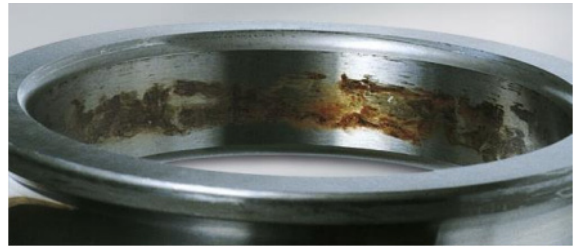
Figure 1: Fretting wear on the inside of bearings.
