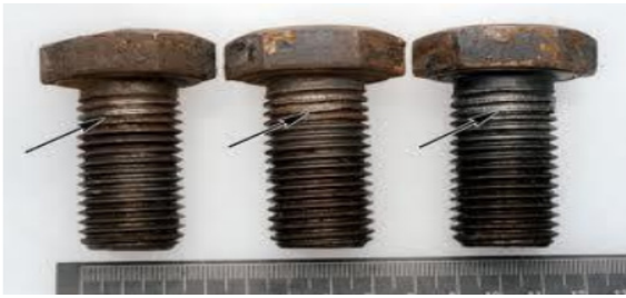
Figure 2: Fretting of threads in bolts.
