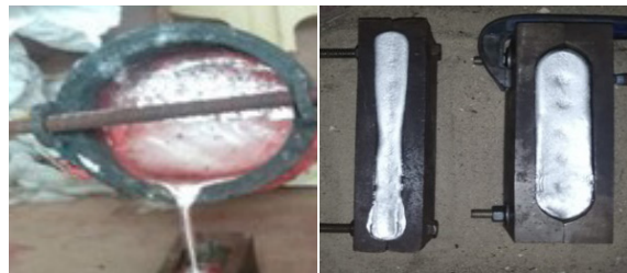
Figure 3: Pouring molten metal.
