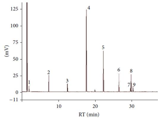
**Figure 6:** Gas chromatography of FAME of extracted oil from copra [29].
