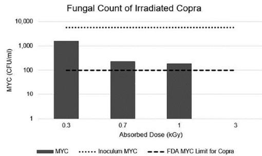
**Figure 1:** Molds and yeast count in copra at different absorbed doses [17].
