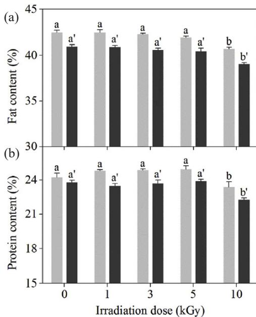
**Figure 3:** Fat and protein contents of irradiated peanut samples at different irradiation doses [28].
