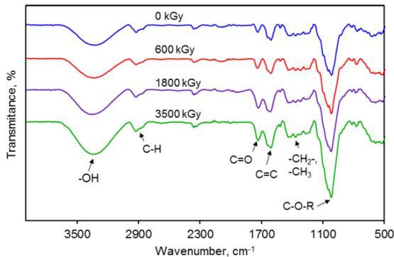
**Figure 4:** FTIR analysis of irradiated orange peel at high absorbed doses [37].
