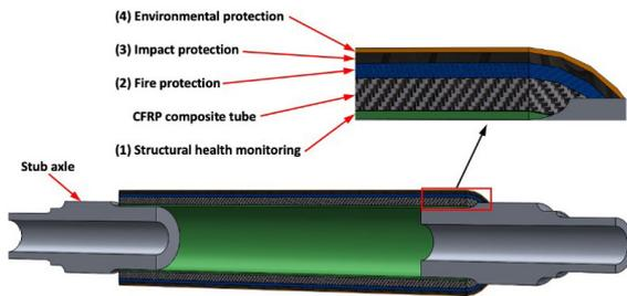
**Figure 3:** Cross-section of a design principle for the hybrid metallic composite railway axle with axial and coaxial skins [36].
