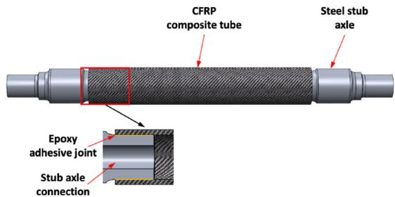
**Figure 2:** Structure of unoptimized structural hybrid metallic-metallic-based composite railway axle principle [36].
