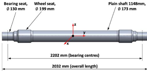
**Figure 1:** An outer part bearing trailer axle with general dimensions [36].
