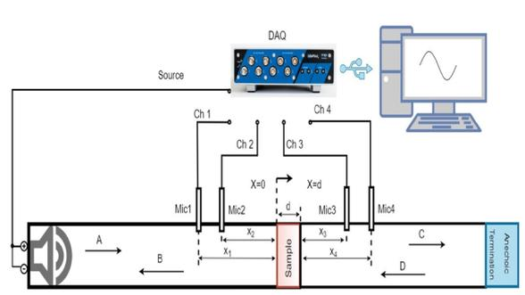
**Figure 2:** Schematics of STL measuring set-up [5]. Reproduced from [5] with permission from Elsevier.
