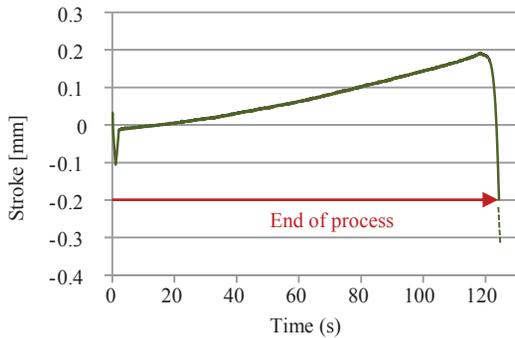
**Figure 11:** Stroke development versus time; Gleeble system was programmed to terminate heating as soon as stroke values fell below  $-0.2$  mm.
