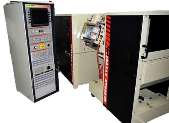
**Figure 2:** Thermo-mechanical simulator Gleeble 3800c (Dynamic Systems Inc.) with control unit (left) and tension/compression module (right).
