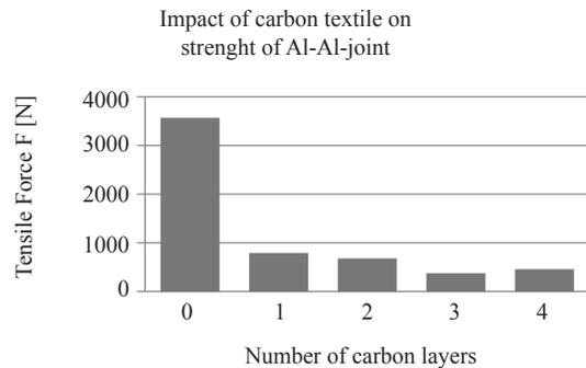
**Figure 14:** Weakening effect of carbon layers on aluminium-aluminium joint.
