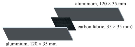
**Figure 4:** Dimension of sample made of carbon fabric (35 × 35 mm) and Al-sheets (120 × 35 mm).
