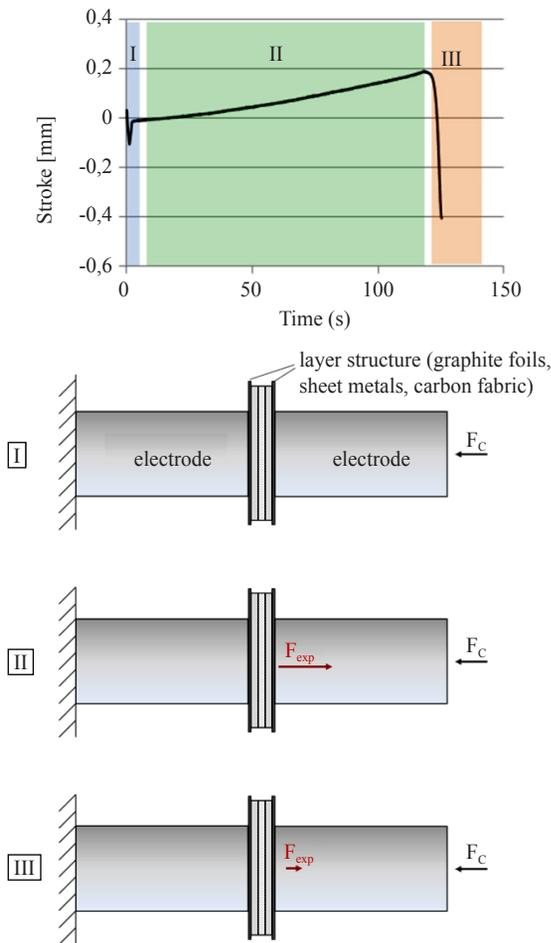
**Figure 9:** Stroke development during heating process and scheme of forces at work.
