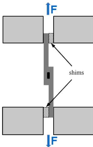
Figure 16: Projected setup of future tensile shear tests.
