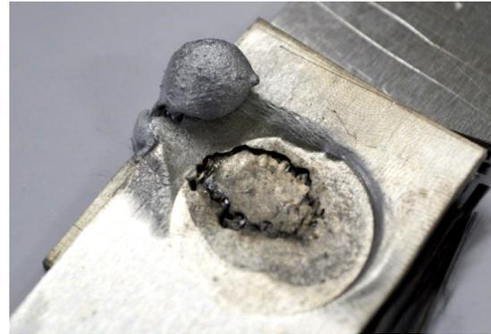
**Figure 13:** Sample with 4 carbon layers, while metal drop on sheet surface emerges as result of poorly penetrable carbon package.
