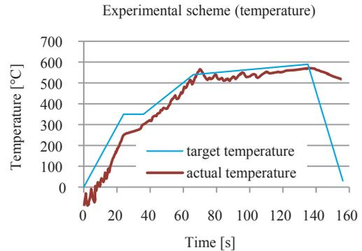
**Figure 7:** Time-Temperature-Diagram depicting targeted and measured temperature development [5].
