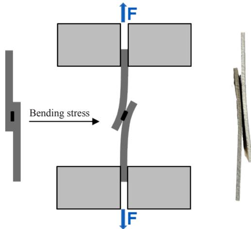
Figure 15: Peeling effect during tensile shear tests.
