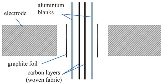
**Figure 3:** Experimental setup consisting of electrodes, aluminium sheets, carbon layers of woven fabric and graphite foils.
