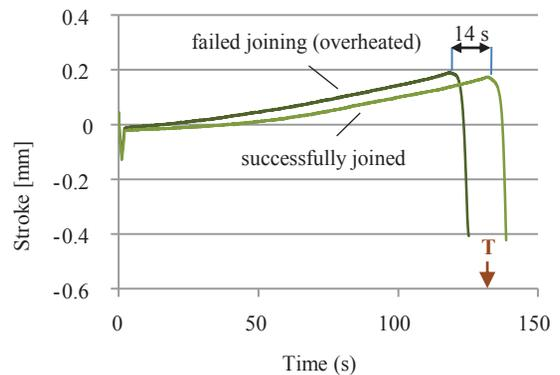
**Figure 10:** Divergent stroke development of two samples being manufactured by identical process parameters (process time  $T = 130$  s).
