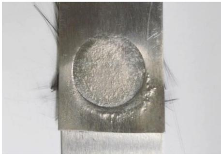
**Figure 12:** Successfully joined sample by stroke-dependent heating process.
