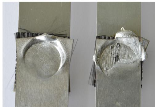
**Figure 8:** Samples indicating substantially different joining results despite of identical process parameters: successfully joined hybrid structure (left); failed sample due to overheating (right). Back sides look similar to front sides.
