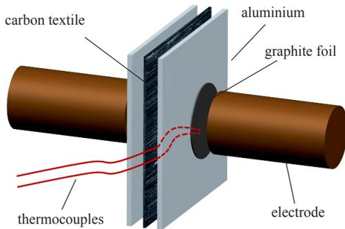
**Figure 6:** Experimental setup revealing welded thermocouples.
