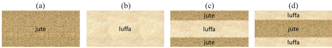
Figure 1: Designs of the test samples: green homogeneous (a) jute and (b) luffa fiber samples, and their hybrid (c) jute-luffa-jute (JLJ) and (d) luffa-jute-luffa (LJL) fiber samples.
