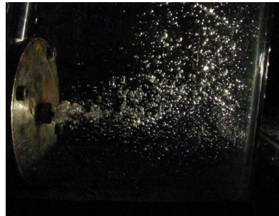
(c) X=1.2 and Q_c=58 \times 10^{-6}\text{m}^3/\text{s} and Q_s=42 \times 10^{-6}\text{m}^3/\text{s} , Shutter speed = 1/2500s
