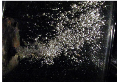
(a) X=0.8 and Q_c=56 \times 10^{-6}\text{m}^3/\text{s} and Q_s=82 \times 10^{-6}\text{m}^3/\text{s} , Shutter speed = 1/2500s
