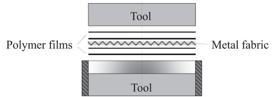
**Figure 2:** Schematic drawing of the cylindrical tool and a single reinforcement layer laminate build up.
