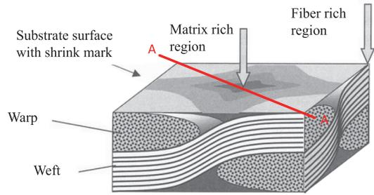
**Figure 4:** Cause of surface texture through local variations in fiber volume fraction and different coefficients of thermal expansion for matrix and fiber.
