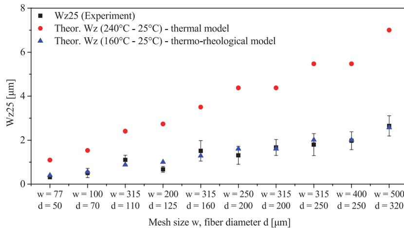
**Figure 11:** Waviness comparison between experimental results and analytical calculated waviness values for different fiber diameter and mesh size combinations.
