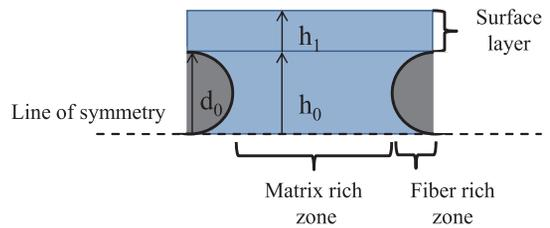
**Figure 5:** Idealized, diagonal cross-section A-A from Figure 4 with additional surface layer  $h_1$ .
