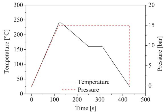
**Figure 3:** Process cycle to manufacture the organic sheets.
