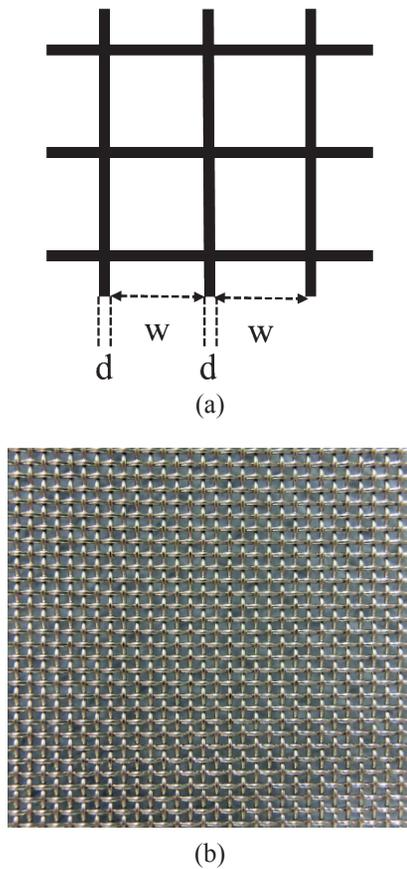
**Figure 1:** (a) Fabric parameters fiber diameter  $d$  and mesh size  $w$ , (b) Example of a plain weave steel wire fabric.
