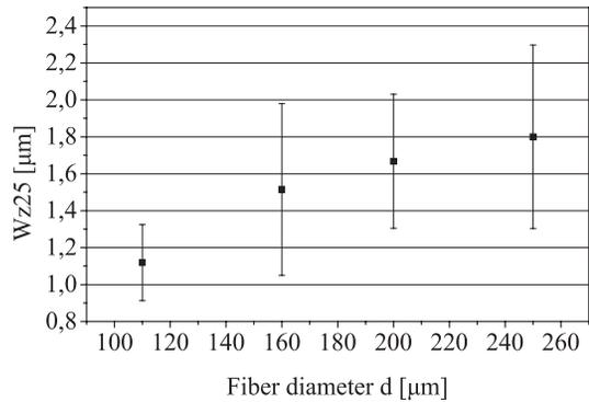
**Figure 8:** Maximum waviness Wz25 in dependency from fiber diameter at a constant w = 315 µm.
