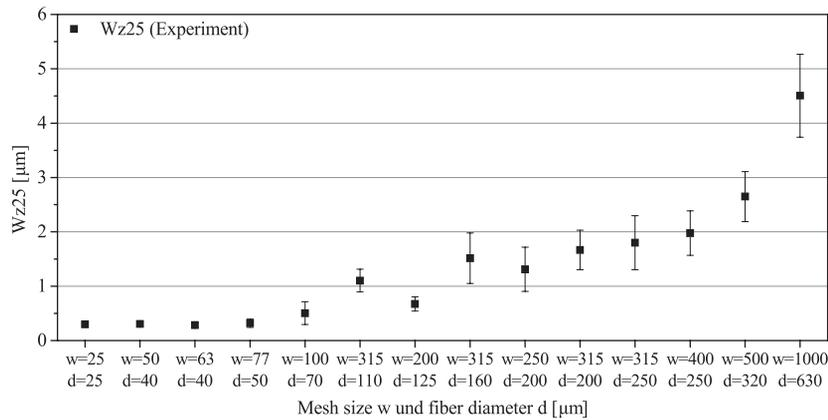
**Figure 7:** Maximum waviness Wz25 in dependence from fiber diameter d and mesh size w for 14 different steel wire fabrics.
