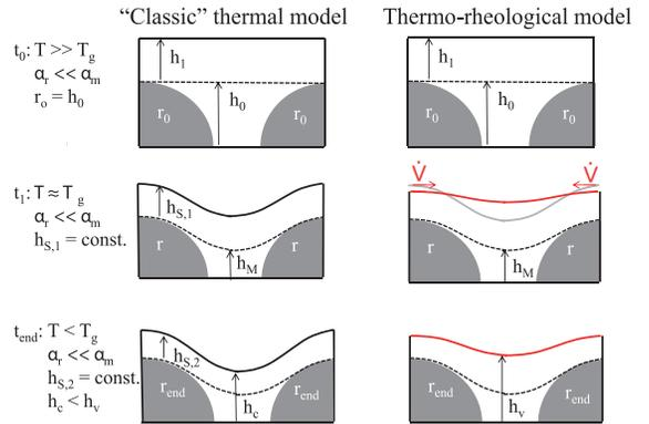
**Figure 10:** Comparison of surface development during processing between thermal and thermo-rheological model.
