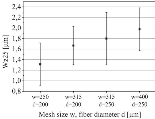
**Figure 9:** Maximum waviness Wz25 in dependency of the mesh size w at two constant fiber diameters.
