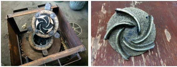
Figure 14: The impeller from vertical centrifugal casting.
