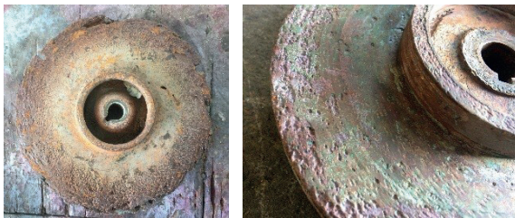
Figure 2: Impellers for seawater pumps after usage.
