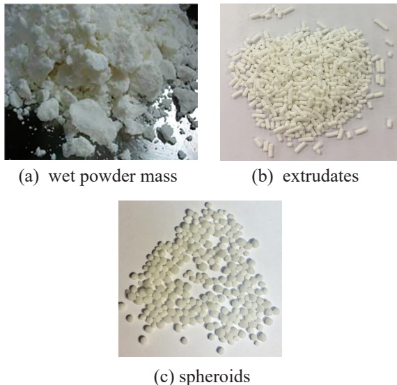
(a) wet powder mass (b) extrudates (c) spheroids Figure 2: The product of extrusion/spheronization process.
