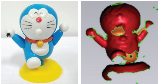
Figure 21: 3D Laser Scan Error (Master model-Left, Scanned Model-Right).
