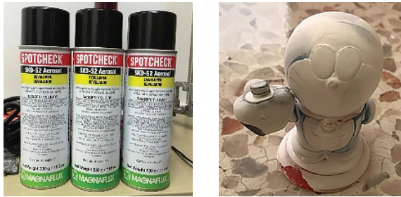
Figure 7: Surface Preparation: (a) White Powder Spray, (b) Coated Master Part.
