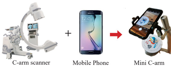
Figure 9: The concept of mini c-arm rotational camera station.
