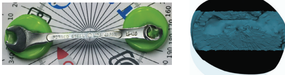
Figure 22: Error due to Defocus (Left), Error due to High Light Intensity (Right).
