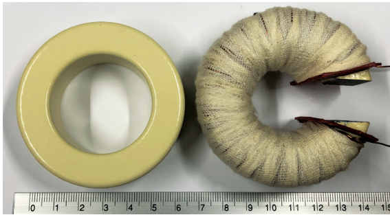
Figure 5: The ferrite core before the cut (left) and finished DC electromagnet coil (unit: cm).
