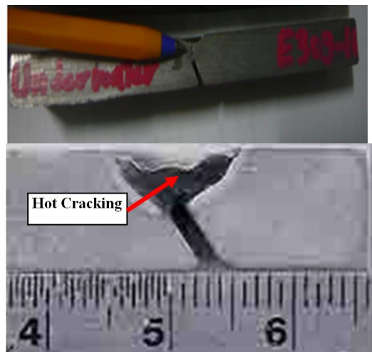
Figure 8: Illustrate of weld hot cracking when used E309-16 electrode, (Nital 2% Etching)
