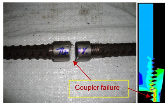
Figure 3: Breaking stress of DB16x3 with coupler diameter of 30 mm (Tighten length of 70%).
