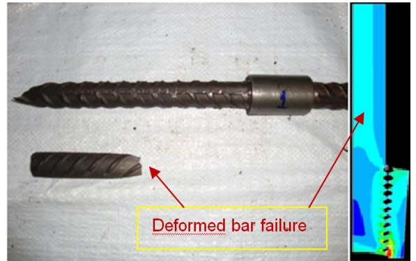
Figure 7: Breaking stress of DB25x3 with coupler diameter of 38 mm (Tighten length of 100%).
