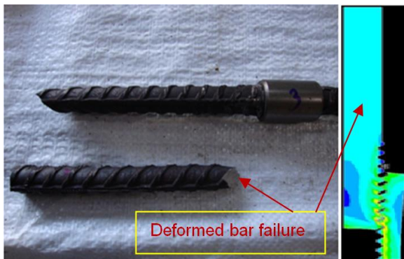
Figure 6: Breaking stress of DB20x2.5 with coupler diameter of 30 mm (Tighten length of 70%).
