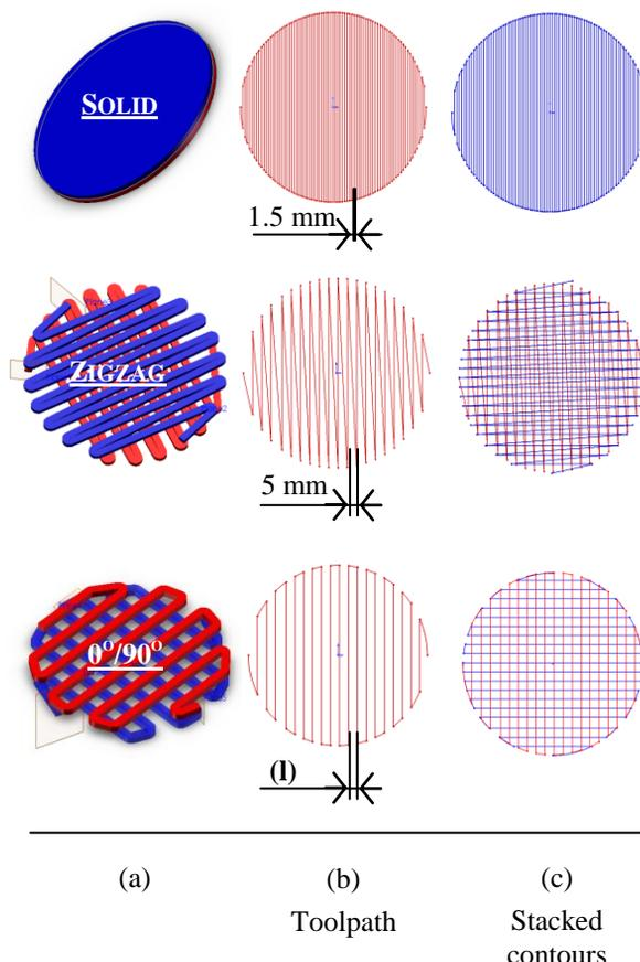
Figure 2: Design of scaffold architectures
