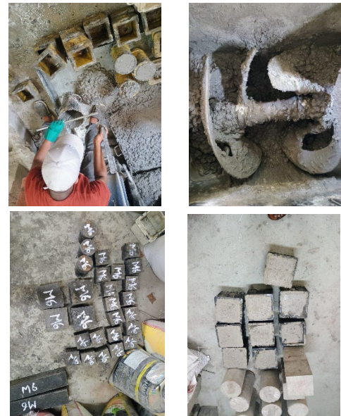
Figure 1: The casting of concrete and samples.
