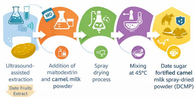
Figure 6: Process representation of encapsulation date sugar camel milk powder production using spray-drying technique.
