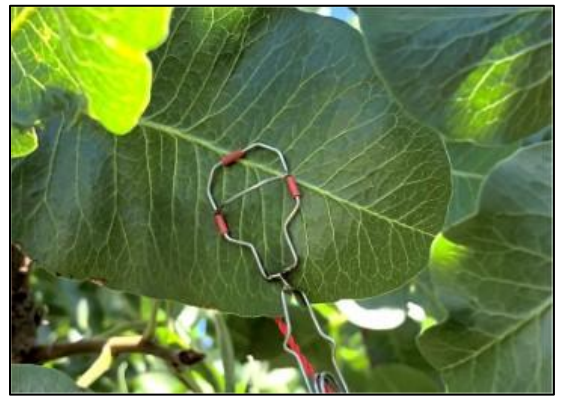
Figure 1: LT-1M leaf temperature sensor (Thermistor type), which measures leaf surface temperature with high sensitivity and stability, providing accurate data for assessing crop water stress in precision irrigation systems.
