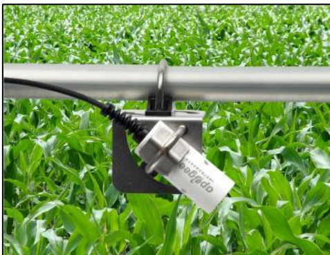
Figure 2: MI-220 leaf temperature sensor (Infrared thermometer), which captures non-contact leaf and canopy temperature readings, enabling continuous monitoring of plant water status in field and greenhouse conditions.
