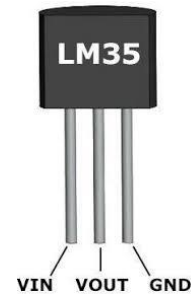
Figure 4: LM35 temperature sensor labelled as VIN (Voltage Input), VOUT (Voltage Output), and GND (Ground), used for direct leaf temperature measurement because of its low cost, accuracy, and linear output.
