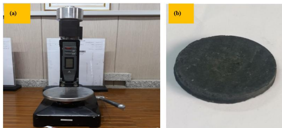
Figure 4: Hardness test setup. (a) Digital durometer conducts shore hardness tests according to ASTM D 2240, (b) Sample.
