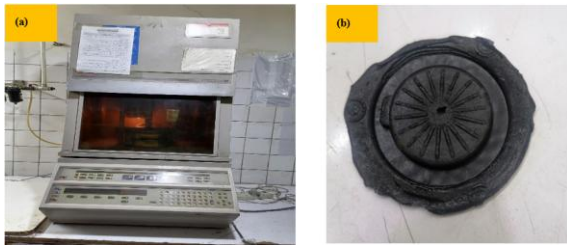
Figure 5: Tests for Cure characteristics (a) Monsanto Rheometer (ODR-2000) and Test specimen after the testing (b) Sample after the test.
