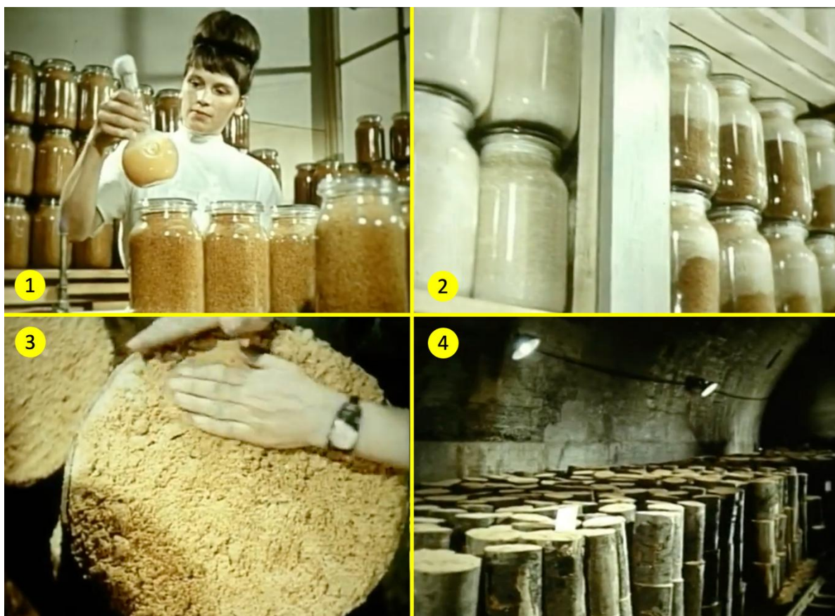
Figure 3: Beech logs bio-modification: (1) Inoculation of sterile substrate: A lab technician fills jars with sterilized sawdust and introduces a fungal spore solution to initiate the mycelium colonization process under controlled conditions; (2) Mycelial colonization phase: Rows of jars containing sawdust show varying stages of white fungal mycelium growth, indicating successful substrate colonization in an incubation room; (3) A fungal substrate is applied to the surface of each beech log, allowing the mycelium to permeate the wood and form fungal networks that alter its characteristics. The logs are then inspected for consistency and uniform fungal colonization before further processing. (4) Fungal maturation in a controlled abandoned bomb shelter in East Germany: Colonized wooden logs are stored in a climate-controlled underground facility, allowing the mycelial structure to stabilize and further develop before industrial use, ©Manfred Beyer, Hans-Günther Kunkel [26].
