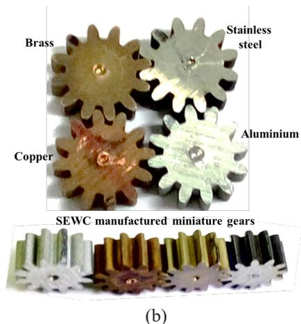
**Figure 2:** (a) Detailed dimensional specifications and different views of the miniature spur gears; and (b) actual SEWC manufactured gears from different materials.
