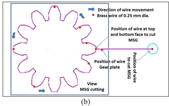
**Figure 4:** (a) Cutting of miniature spur gear by SEWC; and (b) Layout of miniature spur gear.
