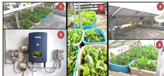
Figure 9: Photographs showing experimental setup (Legends: 1) Cultivated spinach crops below the PV module, 2) Fully grown spinach crops, 3) View of conventional plant, 4) Agrophotovoltaic system, and 5) ACDB, DCDB, Inverter and energy meters).
