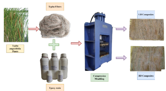
Figure 1: Extraction and manufacturing of TFR composites.
