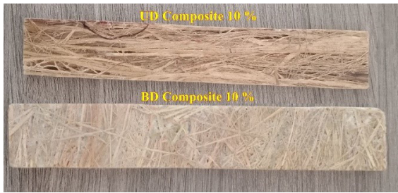
Figure 3: TFR composite specimens for compression test.
