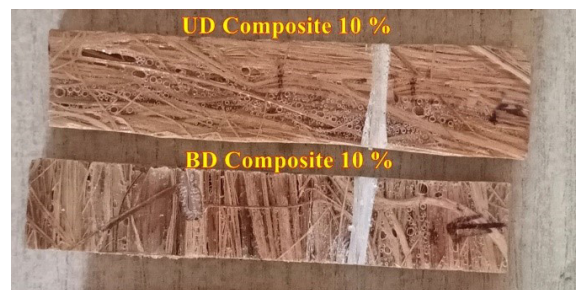
Figure 2: TFR composite specimens for impact test.
