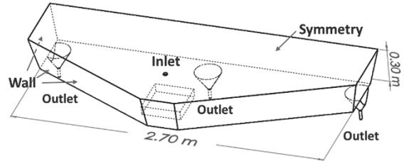
**Figure 5:** Geometry and boundary conditions of the 3-strand tundish model.
