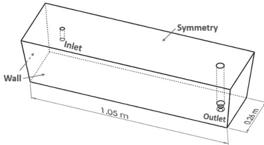
**Figure 3:** Geometry and boundary conditions of the 1-strand tundish model.
