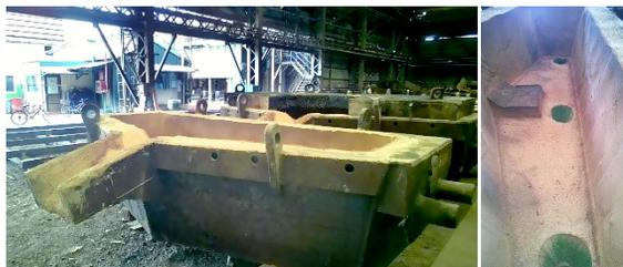
**Figure 2:** Example of the 3-strand continuous casting tundish in the steelwork at BSI, Thailand.
