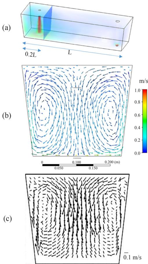
**Figure 8:** (a) Velocity flow field at the plane 0.2L (b) Numerical result from the current study (c) Experimental result from the article [6].
