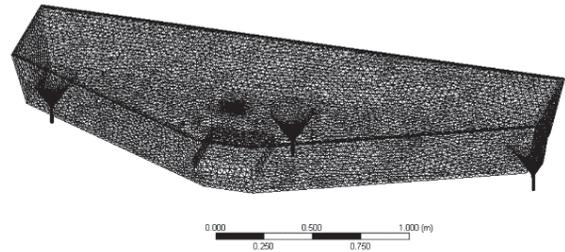
**Figure 6:** Mesh for the 3-strands tundish model.
