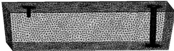
**Figure 4:** Mesh for the 1-strand tundish model.
