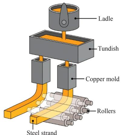
**Figure 1:** Diagram of continuous casting process [1].
