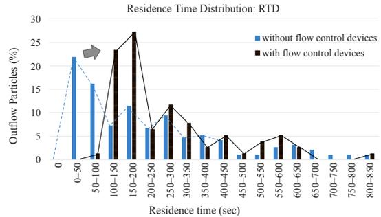
**Figure 11:** Inlet-to-outlet residence time distribution (RTD) of the flow in three-strand tundish model with and without flow control mechanisms.
