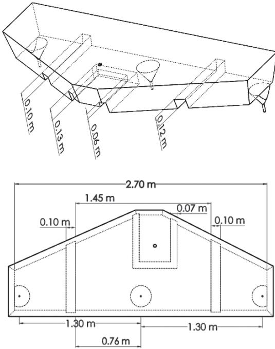
**Figure 7:** Geometry of the designed tundish with flow control mechanisms in 3-D view and top view. The details of geometry, boundary conditions and parameters are shown in Table 2.
