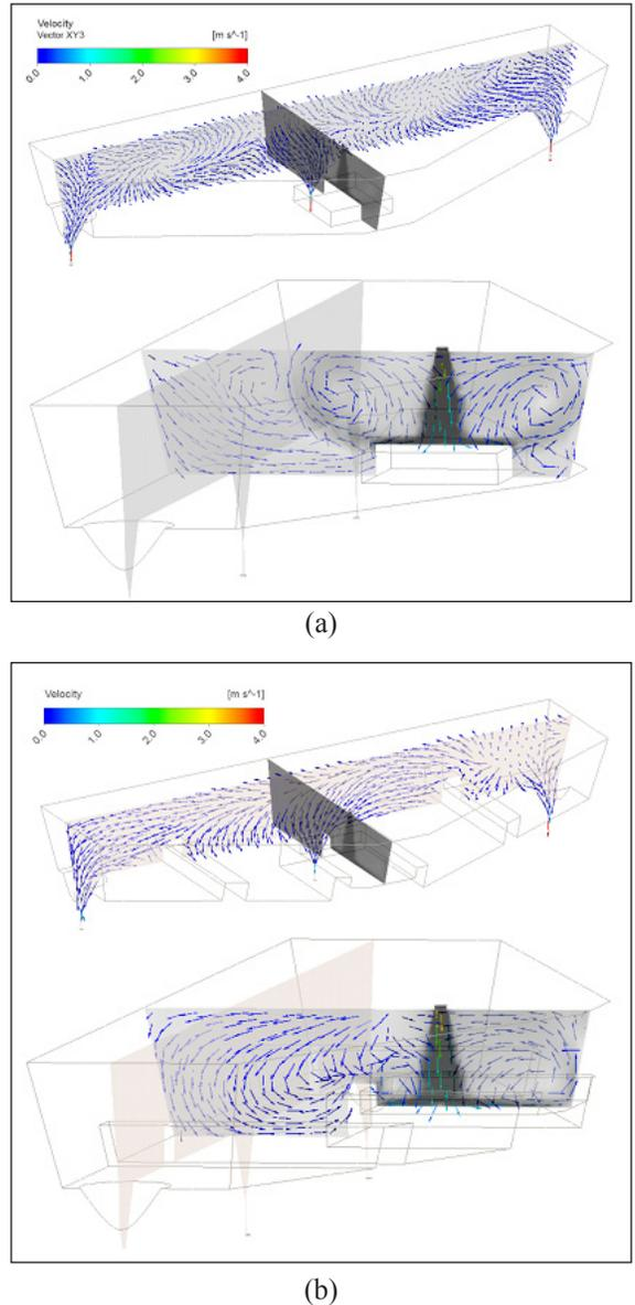
**Figure 9:** Velocity flow field in the three-strand tundish model (a) without flow control mechanisms (b) with flow control mechanisms.
