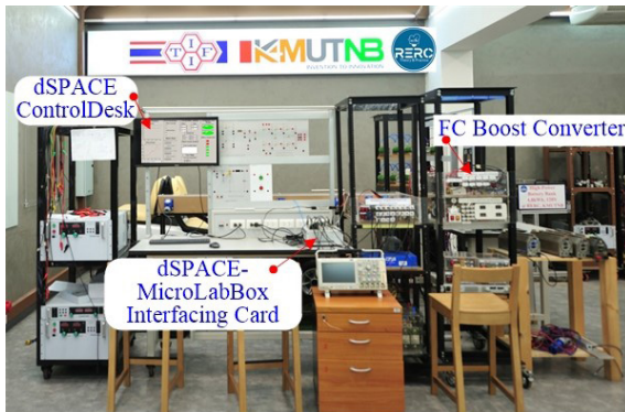
Figure A1: Laboratory experimental test bench of the DC microgrid platform.
