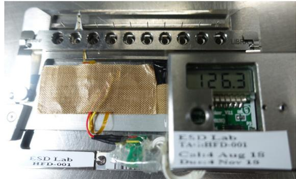
**Figure 6:** Equipment used to measure the copper coil temperature inside a slider.
