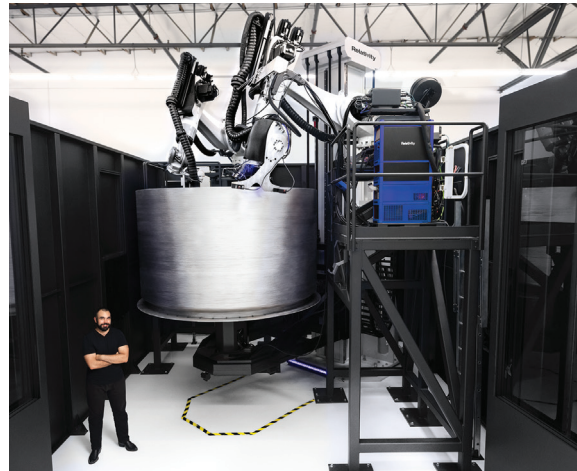
Figure 3: Relativity's Large Format Metal Stargate 3D Printing System producing a Terran 1 first stage tank section.
