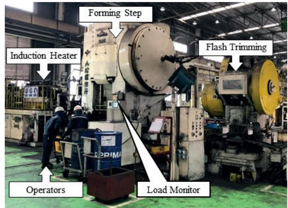
**Figure 7:** The schematic photo of experimental hot forging tests of the talar body prosthesis.
