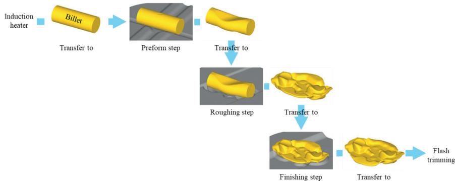
**Figure 3:** Forming steps in the hot forging process of the talar body prosthesis.
