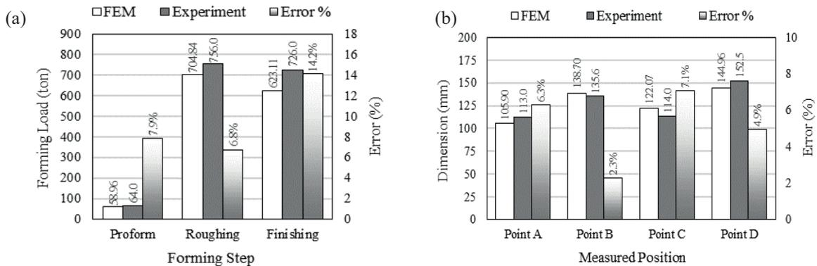
**Figure 9:** Comparison between the FEM and the experimental results in the hot forging process of the talar body prosthesis (a) The forming load errors, and (b) The geometrical errors.
