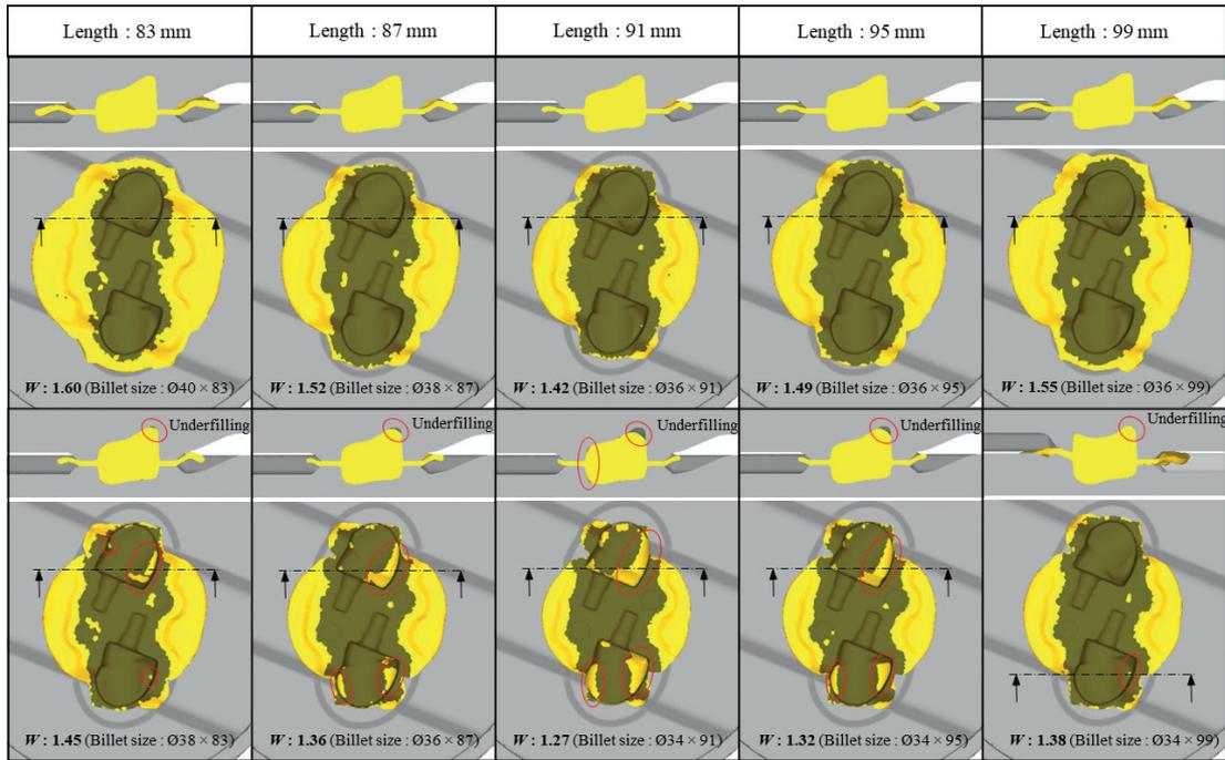
Figure 5: Comparison of the finished forging part at the last step in the FEM.
