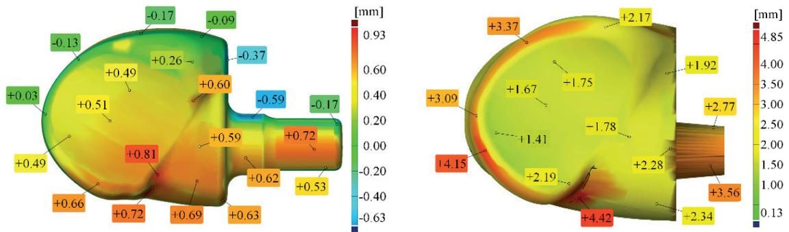
**Figure 10:** Dimensional deviation between the finished forging part and the 3D model (a) 3D Model of the finished forging part, and (b) 3D Model of the talar body prosthesis.
