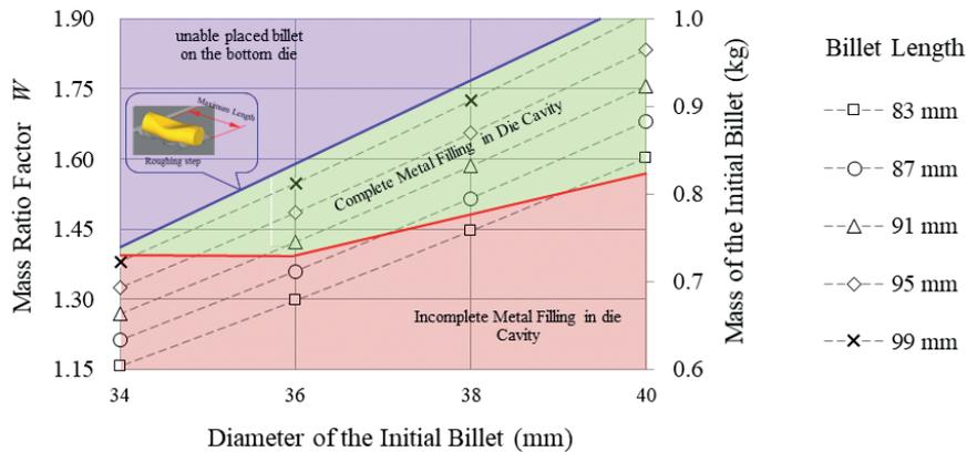
**Figure 6:** Dimension of the initial billet and mass ratio factor limit diagram for the hot forging process of the talar body prosthesis.
