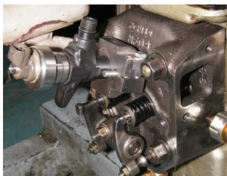
Figure 3: CR injector mounted on modified cylinder head
