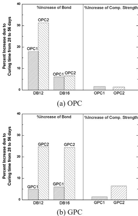
**Figure 5:** Percent increase of bond and compressive strengths due to curing time from 28 to 56 days.
