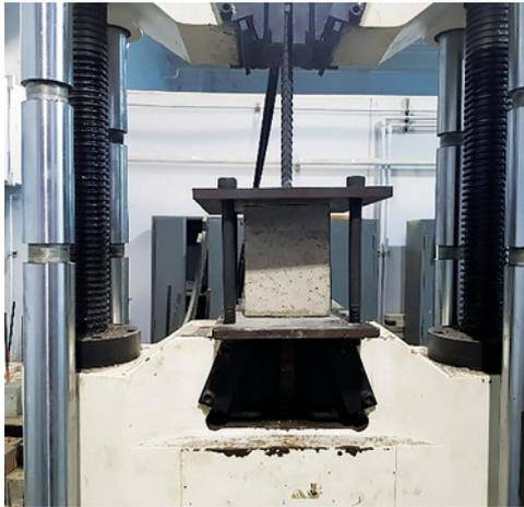
Figure 3: Pull-out test on specimen.
