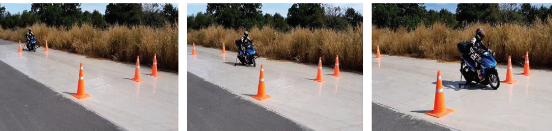
Figure 16: CBS-equipped motorcycle during braking maneuver (from left to right).
