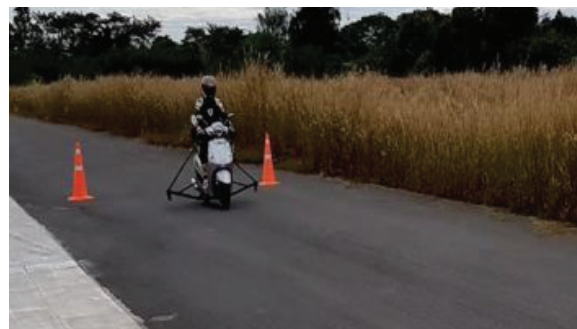
Figure 7: Braking performance test on high friction surface with a nominal peak breaking coefficient of 0.9 (1st Protocol).
