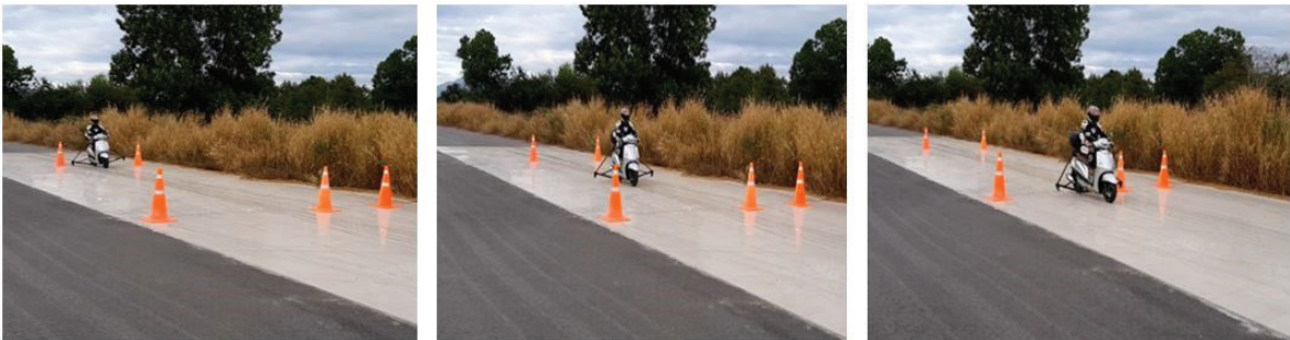
Figure 15: ABS-equipped motorcycle during the braking maneuver (from left to right).
