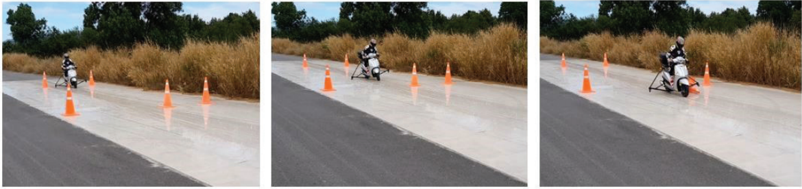
Figure 14: Non-ABS-equipped motorcycle during the braking maneuver (from left to right).
