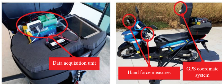
Figure 6: Installation of measurement Units in test motorcycle.
