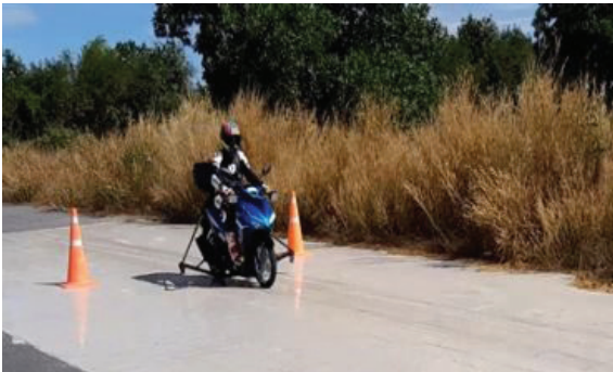
Figure 8: Braking performance test on low friction surface with nominal peak breaking coefficient of <0.55 (2nd Protocol).
