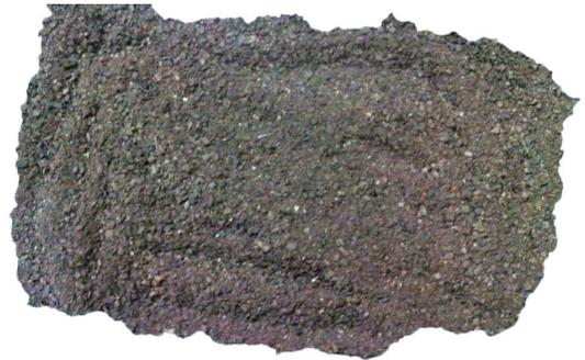
**Figure 4:** Milled plantain peel retained on U.S. standard sieve size number 50 (0.30 mm opening).
