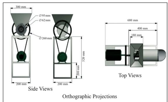
Figure 2: Orthographic projections of the varying die-plate fish feed pelletizer.
