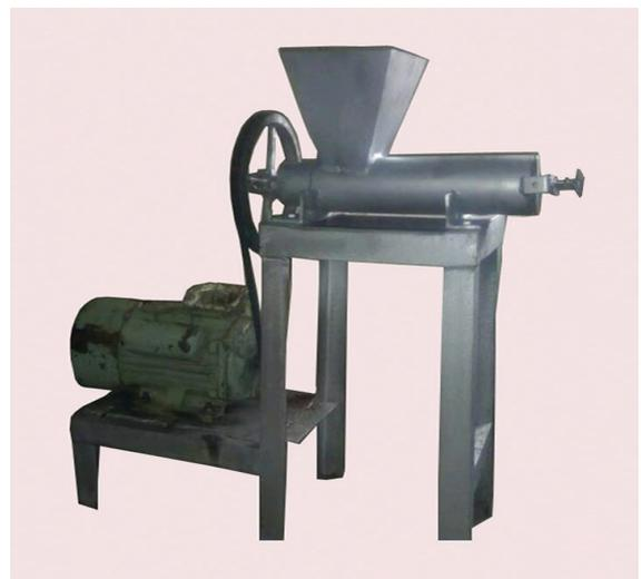
Figure 3: Pictorial view of a varying die-plate fish feed pelletizer.
