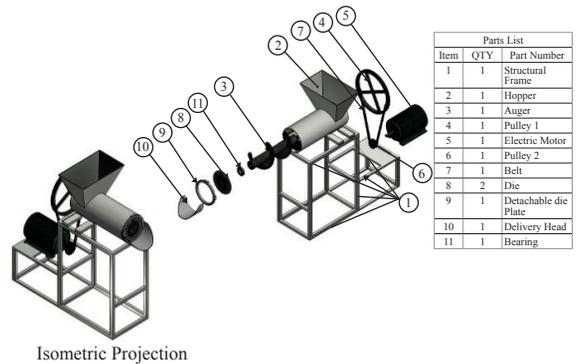
Figure 1: Exploded view of the varying die-plate fish feed pelletizer.
