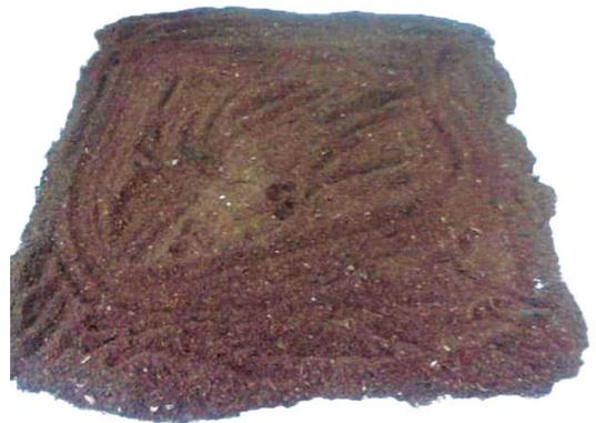
**Figure 5:** Milled citrus peel retained on U.S. standard sieve size number 50 (0.30 mm opening).
