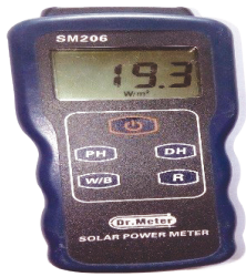
Figure 4: Dr Meter SM206 Solar Power Meter used for the Irradiance data capture.
