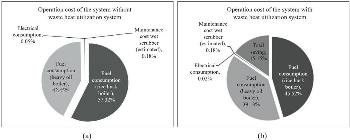
**Figure 10:** Operation cost of the system with and without waste heat utilization system; (a) system without waste heat utilization; (b) system with waste heat utilization.
