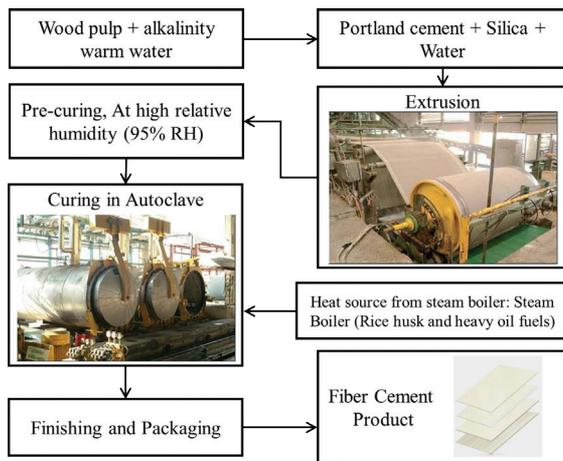
Figure 1: Fiber cement Process diagram [1].
