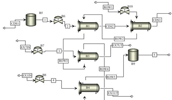
**Figure 7:** Waste heat recovery block diagram from Aspen plus.
