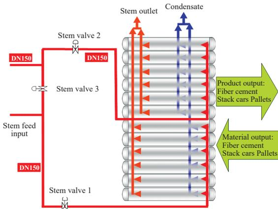
Figure 4: The autoclave system layout.
