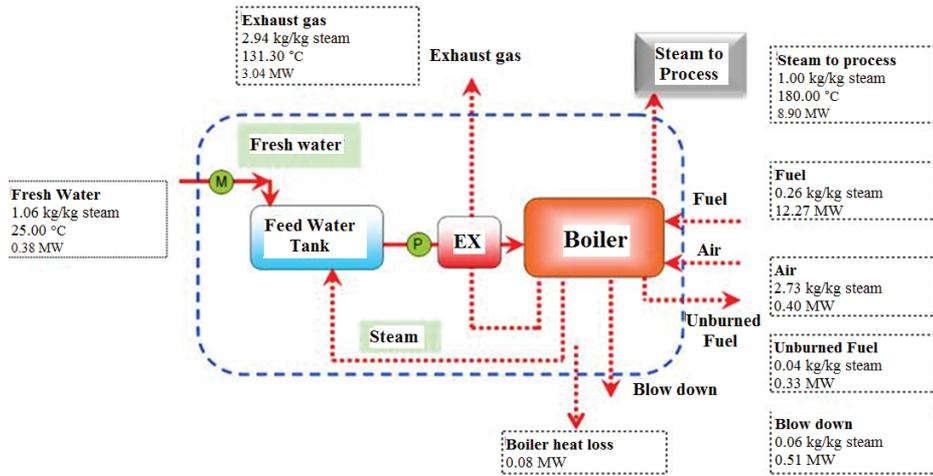
Figure 3: The heat and mass balance diagram of boiler at normal operation.
