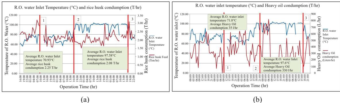
**Figure 9:** The R.O. water temperature before feeding to both boilers with and without waste heat utilization system; (a) The R.O. water temperature before feeding to the rice husk boiler; (b) The R.O. water temperature feeding to the heavy oil boiler.
