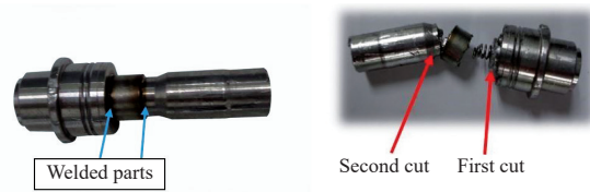
Figure 8: Welded parts being cut to expose and remove inner components.
