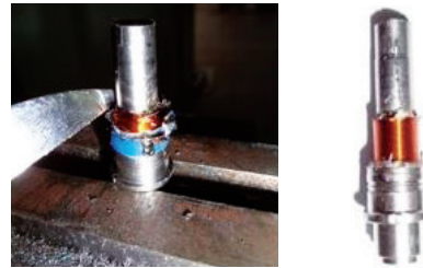
Figure 7: Polymer being removed with a cutting knife after it has been melted.
