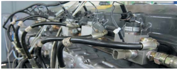
Figure 2: Installation of injector A.
