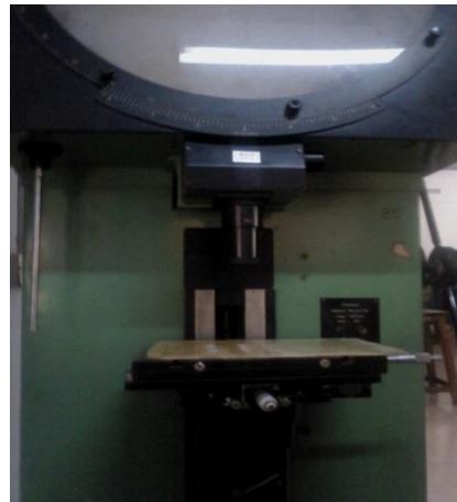
Figure 1: Profile Projector experimental setup for specimen-2 and specimen-3
